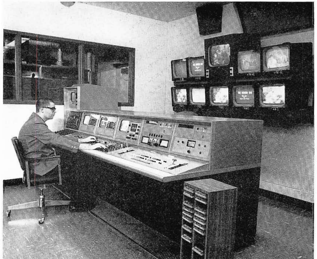
FIG. 3. Operator Dick Clay at the console in master control handles the station breaks while at the same time is able to watch the operation of the transmitter.
