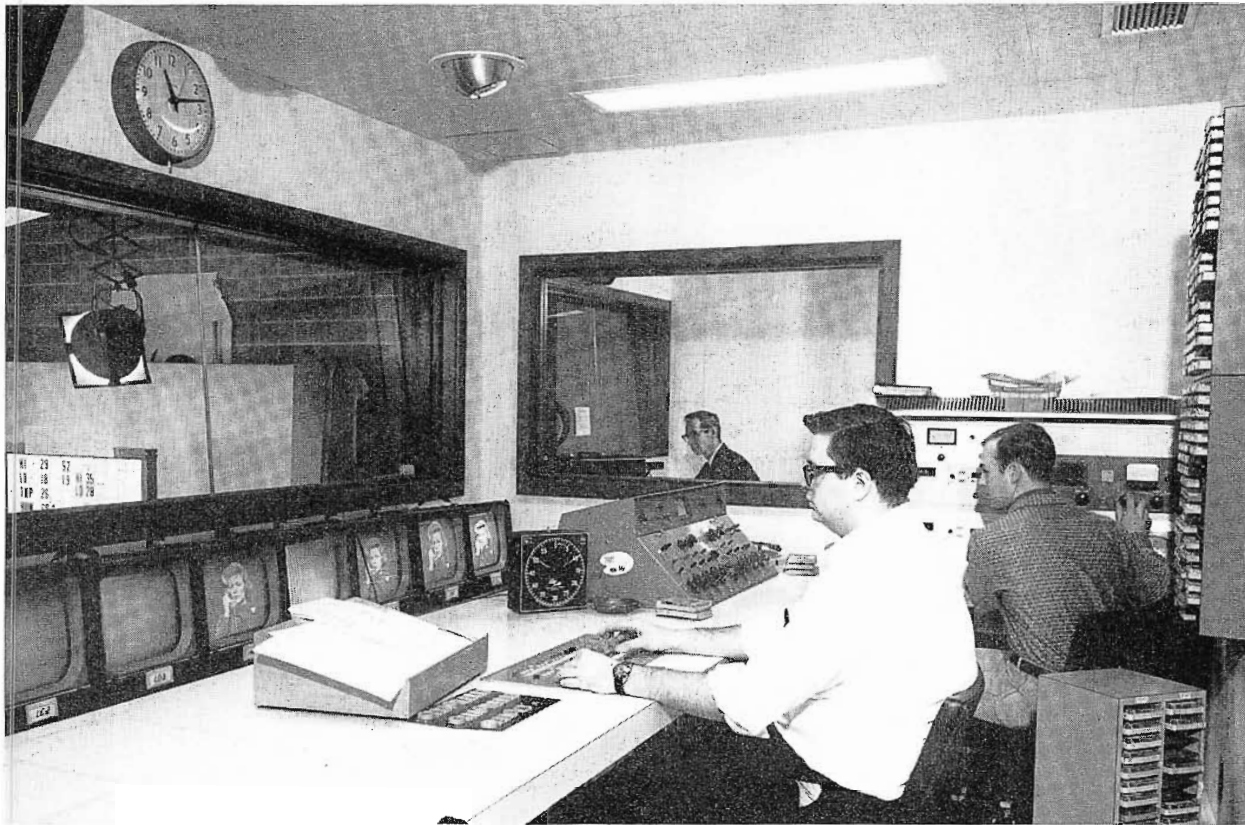
FIG. 8. Studio Control and the announce booth look directly into the studio. Director, Jon Boettcher, does his own switching during live and tape sessions. The audio man has a BC-8 audio console turntable, cartridges and reel recorders at his fingertips. The booth announcer can look into the studio control room or into the studio.
