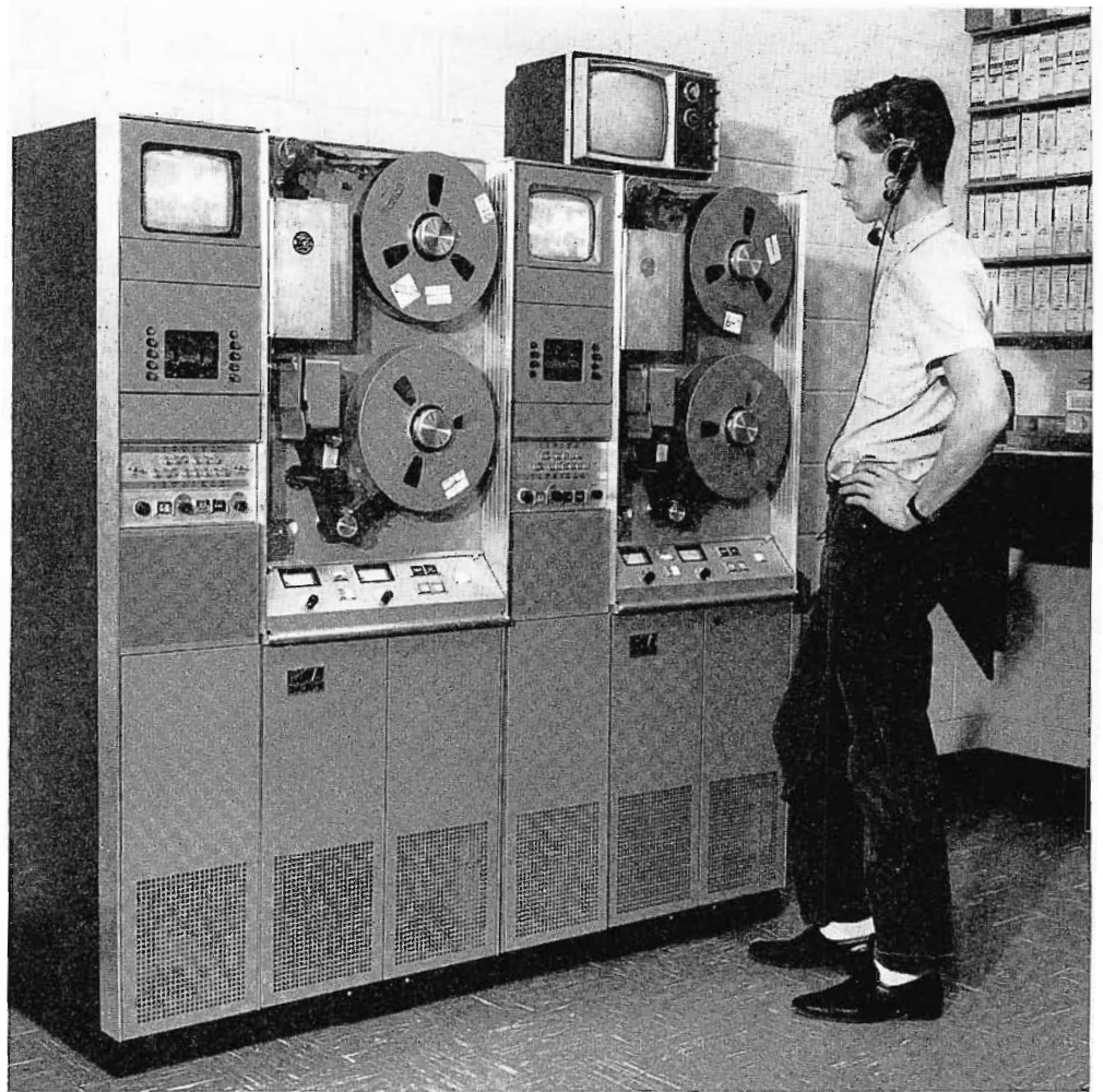
FIG. 6. Due to heavy demand for local production, the record components for the TR-3 were installed after only six months on the air. The machines are equipped to record and play color video tape. Engineer, Dan Wasmund, checks performance.
