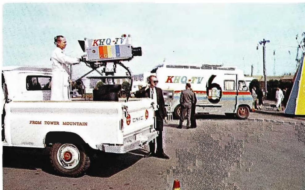
FIG. 4. With a single TK-42 and the TR-5, power requirements were so small that one could move almost at will around the many acres covered by the Fair. By using the electronic splicer on the TR-5, a show was built a section at a time and when played back, had the appearance of multi-camera coverage.
