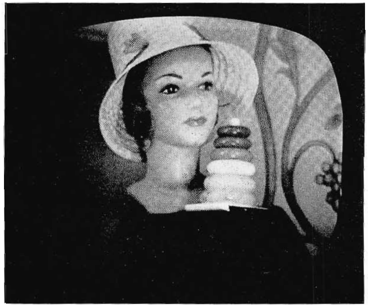
FIG. 4B. Photo of color TV screen showing relative absence of noise when luminance is obtained from noise-free tube.
