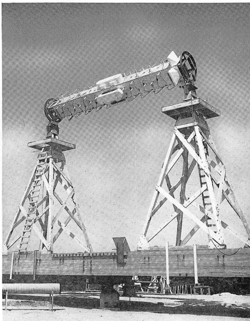
FIG. 3. The Zee Panel mounted high on horses and turntable for radiation pattern measurements. In plotting horizontal circularity patterns, the antenna revolves on the horses. For vertical pattern tests, the entire assembly rotates.
