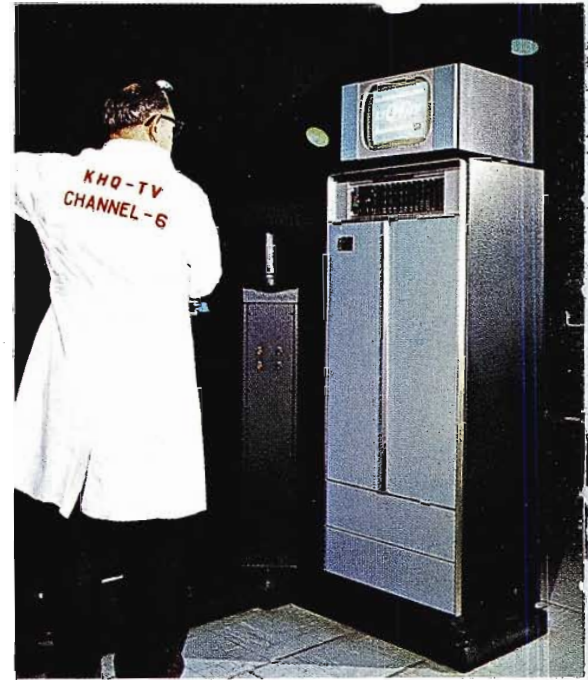
FIG. 8. The RCA TK-27 color film chain installed at KHQ-TV.
