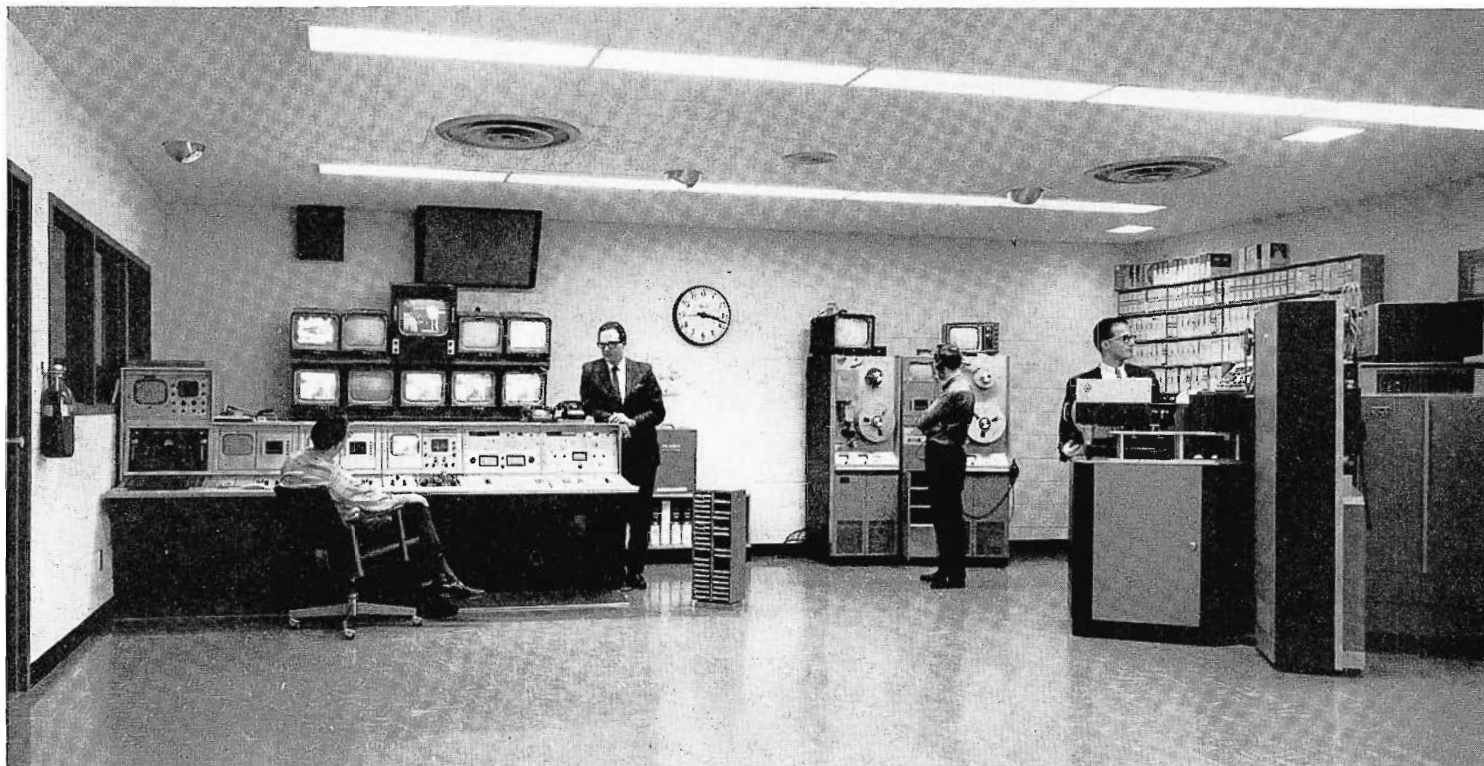
FIG. 1. The WCEE-TV Master Control was planned with switcher, video and cartridge tape machines, film and slide projectors, and camera control units for TK-60 and TK-41 cameras, all located in one room. Since this area is adjacent to the transmitter on the left, it is possible to operate with
